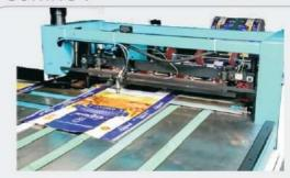
Heat Cut: To cut unlaminated woven fabric with accurate size, which is maintained by Servo System.
