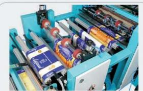
To Reserve Extra Length of Fabric opened during continuous unwinding & maintain uniform tension of fabric
