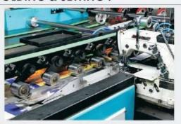
Folder: Single & Double fold type folders. Which is suitable for all type of fabrics. Sewing: Most Suitable Model: AS 102 HS "ARM STITCH" Brand – Ginza make sewing machine.
