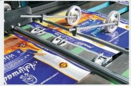
To transfer cutted piece of bag from cutting unit to folding device + sewing unit.
