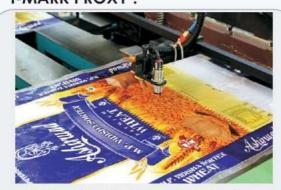
To cut accurate length as per print on fabric.
